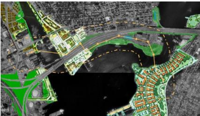
The above ground waterfront power lines (solid yellow line) will be highly visible from projected development parcels in Providence and E. Providence, reducing their property value.
